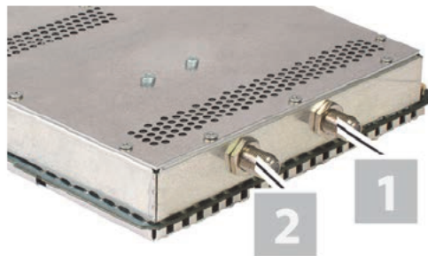
Figure 5: Connecting tuner with DVB-T/T2/C signal
