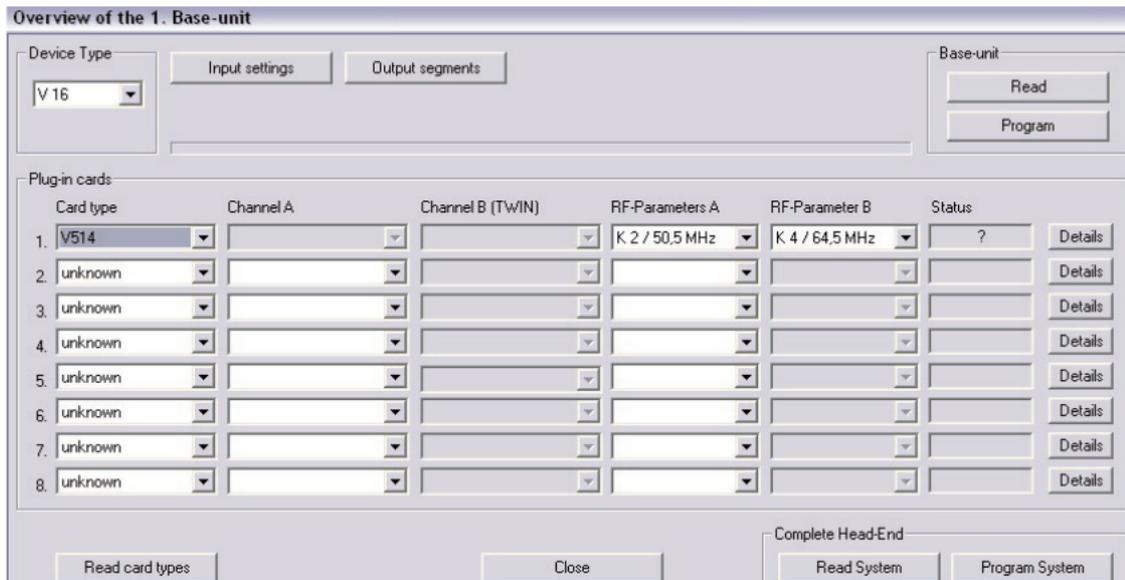
To select the transponders to be received from, you must first define in the basic unit which Satellite-levels are connected. This is done under “Occupy inputs”. The illustration below shows which signals are available at each of the respective inputs.
