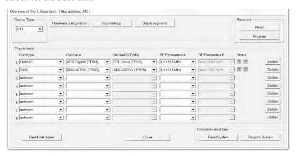
To select the transponders for reception, the satellite levels connected must be defined in the base unit first. This is done under "Feeding of the inputs". The figure below shows which signals are available at the respective inputs.
