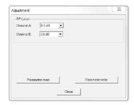
The values currently stored are first read from the card when the "Read parameters" button is clicked. Any modifications made will only be written to the card and activated when the "Parameter write" button is pressed.
