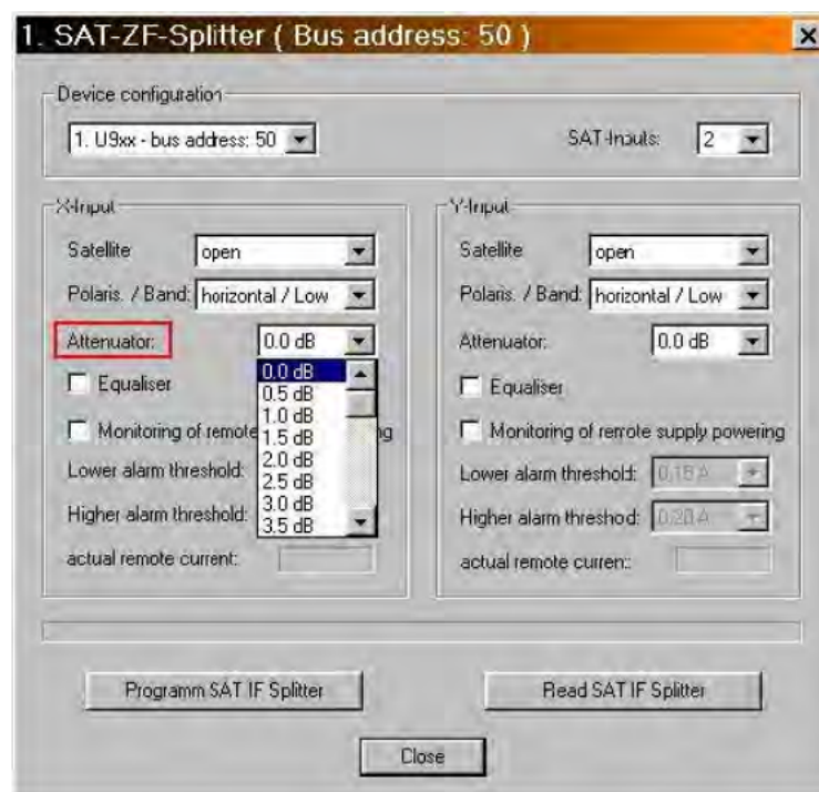
Figure 5: SAT IF splitter, setting the attenuator
