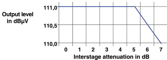
*The output voltage as a function of the interstage attenuation value*
