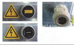
Depending on the part number, the amplifier's power supply connection can either be a flat cable socket or a PE cable gland (see bottom left).
