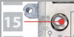
At the input, there is a bidirectional test socket [15] with 20 dB decoupling attenuation. You can use it to:
