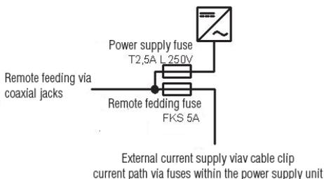
Remote feeding fuses depend on configuration of the device.
