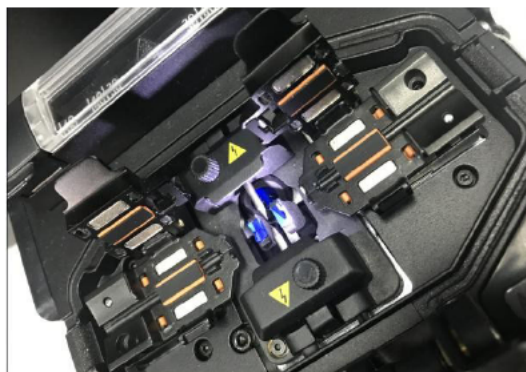
Figure 15: Loading fibre into the splicer
