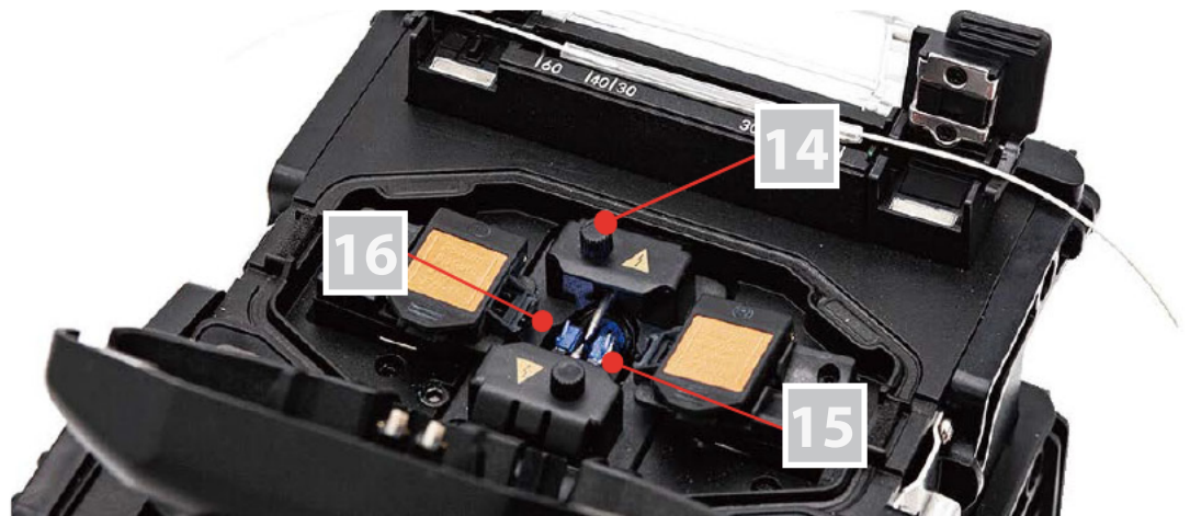
Figure 2: AFS-GS61, wind protection opened
