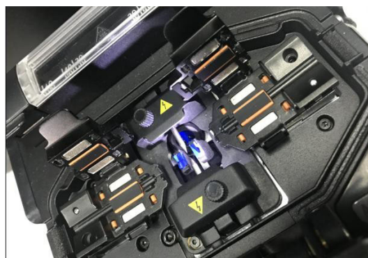
Figure 15: Loading fiber into the splicer
