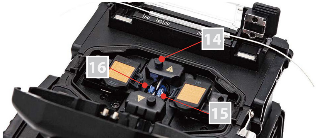
Figure 2: AFS-GS41, wind protection opened
