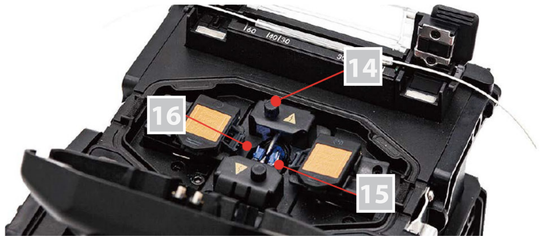
Figure 2: AFS-GS41, wind protection opened
